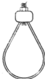
ADJUSTABLE BAND HANGER TYPE - 9
